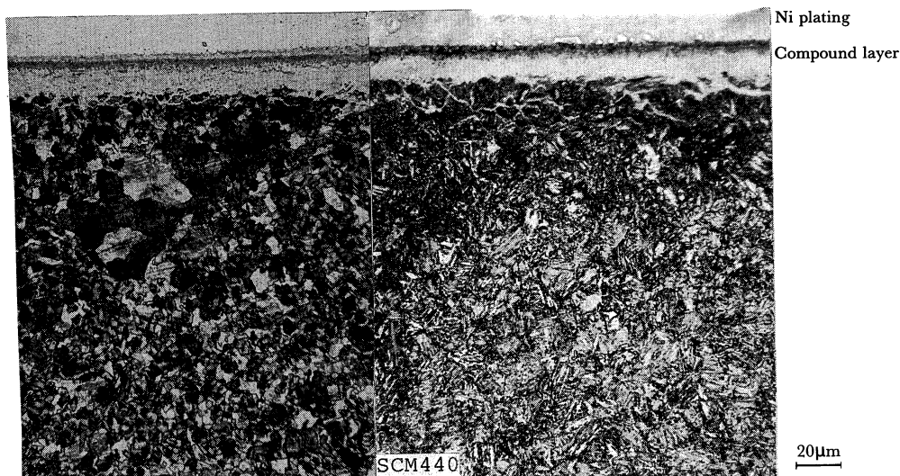
Fig. 2 Cross-sectional microstructures of steels, gas sulfonitrided in a \text{N}_2\text{-NH}_3\text{-H}_2\text{S} atmosphere at 843 K for 14.4 ks.
