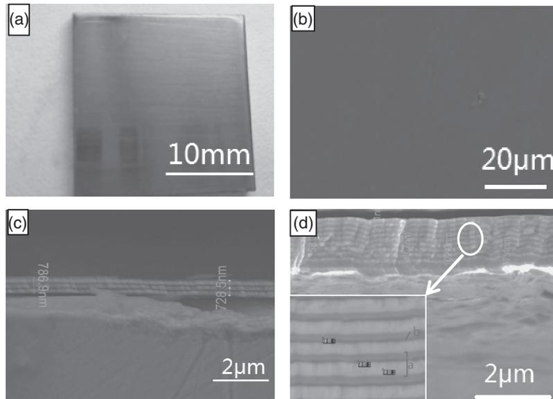
Fig. 1 Microstructure of the films. (a) Sample appearance. (b) Coating surface. (c) Cross-section (3 layers). (d) Cross-section (10 layers).
