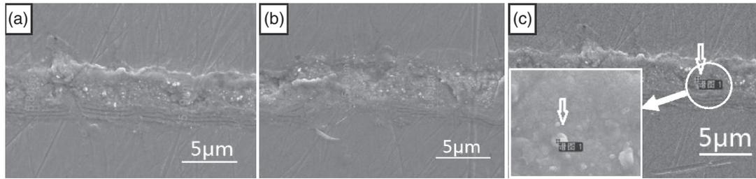
Fig. 3 Micrographs by SEM. (a) Bond with unreacted strips. (b) Fusion zone. (c) Residual nickel particles with EDX.
