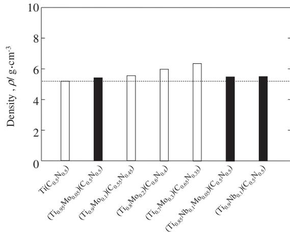
Fig. 1 Densities of the titanium carbonitride substrates. The dash line indicates the true density of Ti(C<sub>0.5</sub>N<sub>0.5</sub>).
