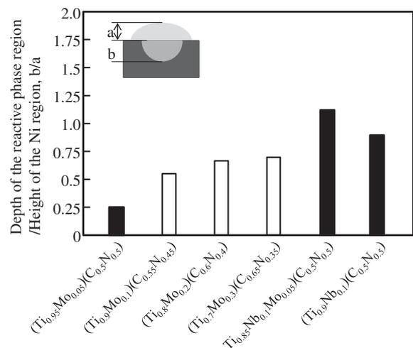
Fig. 7 Ratio of the depth of the reactive region to the height of the Ni region for  $(\text{Ti}_{0.95}\text{Mo}_{0.05})(\text{C}_{0.5}\text{N}_{0.5})$ ,  $(\text{Ti}_{0.85}\text{Nb}_{0.1}\text{Mo}_{0.05})(\text{C}_{0.5}\text{N}_{0.5})$  and  $(\text{Ti}_{0.9}\text{Nb}_{0.1})(\text{C}_{0.5}\text{N}_{0.5})$ ; the schematic illustration of cross section shows  $b/a$  ratio and the previous data for Ni on TiMoCN are superimposed.<sup>18)</sup>
