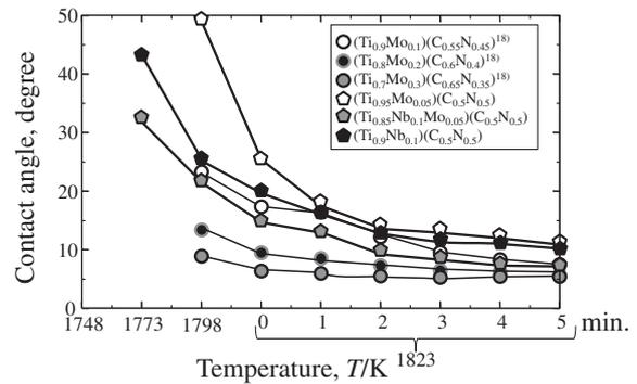
Fig. 3 Contact angle as a function of temperature and holding time for Ni on (Ti<sub>0.95</sub>Mo<sub>0.05</sub>)(C<sub>0.5</sub>N<sub>0.5</sub>), (Ti<sub>0.85</sub>Nb<sub>0.1</sub>Mo<sub>0.05</sub>)(C<sub>0.5</sub>N<sub>0.5</sub>) and (Ti<sub>0.9</sub>Nb<sub>0.1</sub>)(C<sub>0.5</sub>N<sub>0.5</sub>); the previous data for Ni on TiMoCN are superimposed.<sup>18)</sup>
