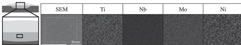
Fig. 6 Schematic illustration of observed cross section, SEM images and EDS mappings of the Ni on  $(\text{Ti}_{0.85}\text{Nb}_{0.1}\text{Mo}_{0.05})(\text{C}_{0.5}\text{N}_{0.5})$  samples after the wetting test. The dashed squares on the SEM images are the regions for which EDS mapping was performed.
