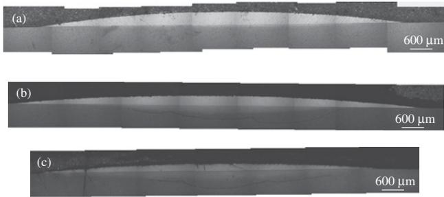
Fig. 4 Optical micrographs of the cross sections of the samples, recorded after the wetting tests: Ni on (a)  $(\text{Ti}_{0.95}\text{Mo}_{0.05})(\text{C}_{0.5}\text{N}_{0.5})$ , (b)  $(\text{Ti}_{0.85}\text{Nb}_{0.1}\text{Mo}_{0.05})(\text{C}_{0.5}\text{N}_{0.5})$  and  $(\text{Ti}_{0.9}\text{Nb}_{0.1})(\text{C}_{0.5}\text{N}_{0.5})$ .
