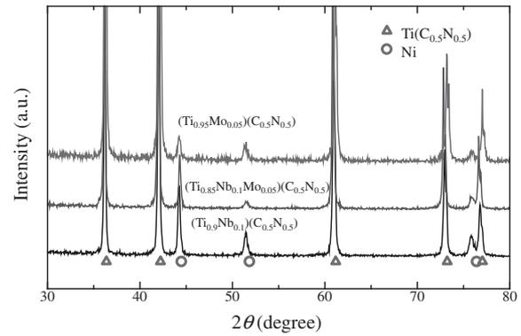
Fig. 5 XRD patterns of the cross sections of the samples, recorded after the wetting tests: Ni on  $(\text{Ti}_{0.95}\text{Mo}_{0.05})(\text{C}_{0.5}\text{N}_{0.5})$ ,  $(\text{Ti}_{0.85}\text{Nb}_{0.1}\text{Mo}_{0.05})(\text{C}_{0.5}\text{N}_{0.5})$  and  $(\text{Ti}_{0.9}\text{Nb}_{0.1})(\text{C}_{0.5}\text{N}_{0.5})$ .
