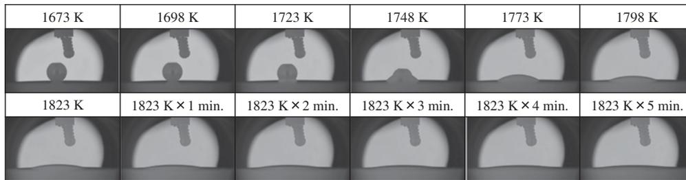
Fig. 2 Photo images of the Ni on (Ti<sub>0.85</sub>Nb<sub>0.1</sub>Mo<sub>0.05</sub>)(C<sub>0.5</sub>N<sub>0.5</sub>) during wetting test.
