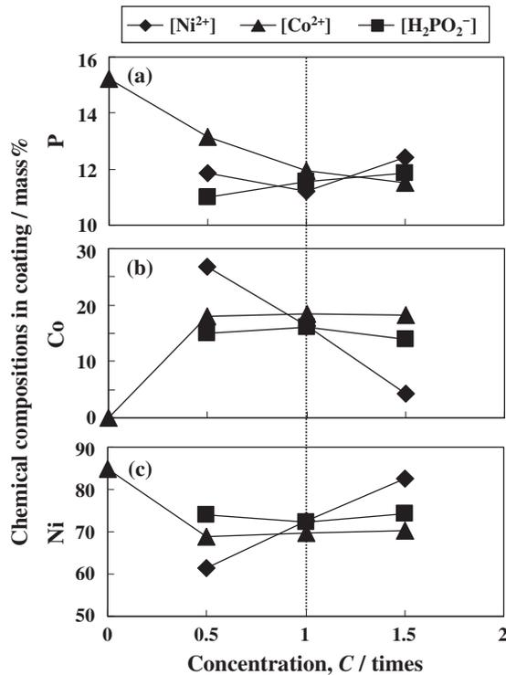
Fig. 2 Effects of ion concentrations of plating bath on coating composition.
