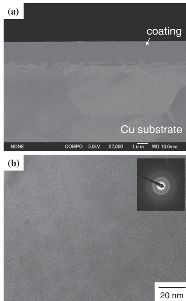
Fig. 1 Observation of Ni–Co–P coating deposited at standard condition: (a) BSE image of polished cross section, (b) TEM in-plane view with diffraction pattern.
