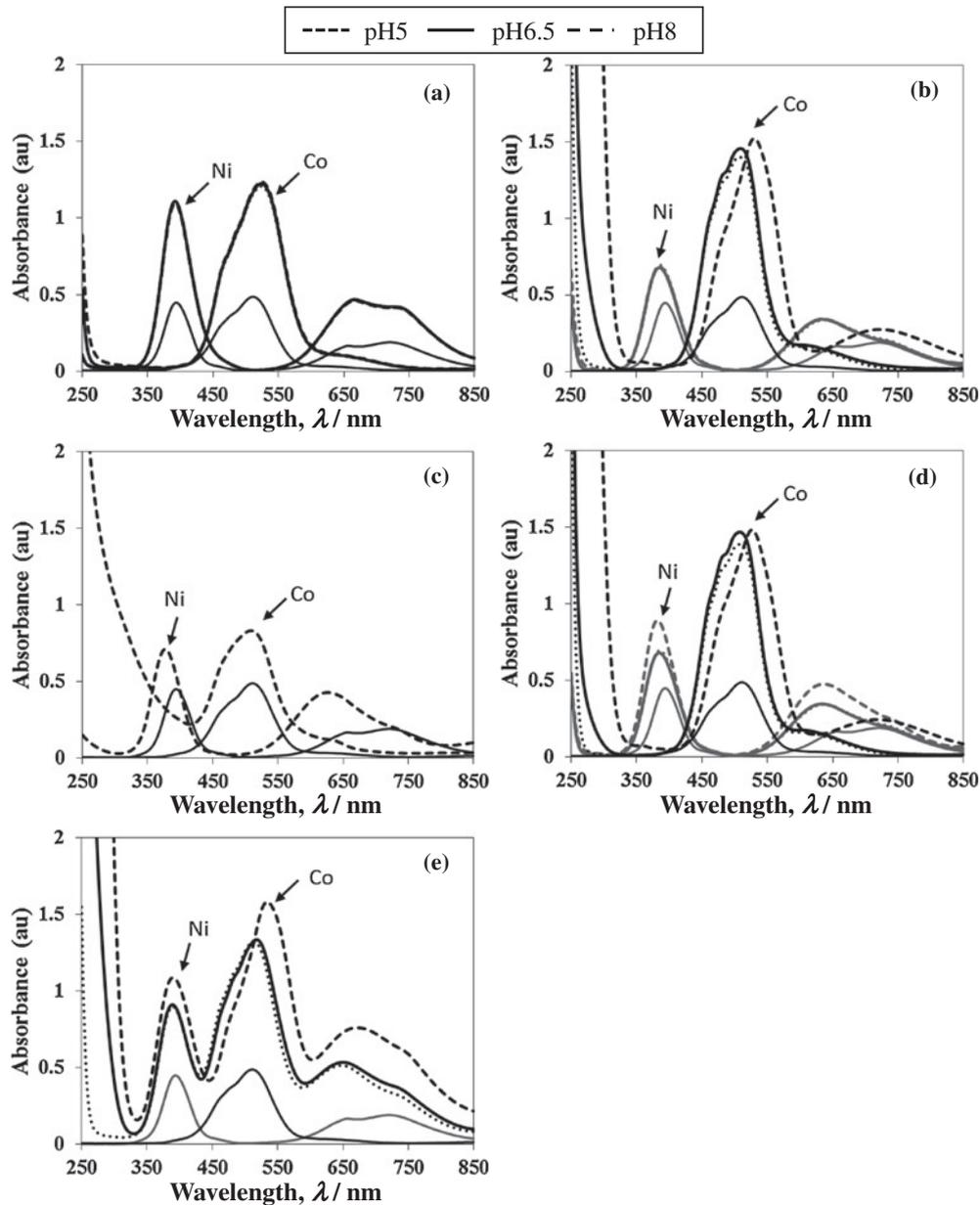
Fig. 6 The UV-vis spectra of nickel and cobalt solution at several pH values with the addition of (a) sodium lactate, (b) sodium citrate, (c) ammonia sulphate, (d) ammonia citrate and (e) plating solution.
