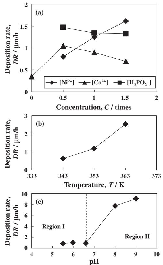
Fig. 5 Deposition rate as a function of (a) ion concentrations, (b) temperature and (c) pH.
