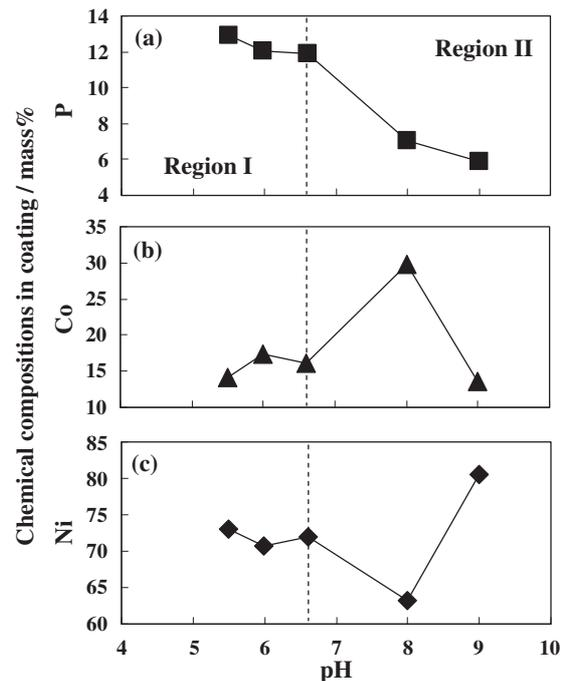
Fig. 4 Effect of pH of plating bath on coating composition.
