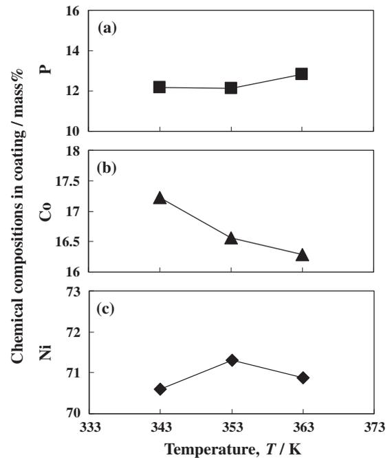
Fig. 3 Effect of temperature of plating bath on coating composition.
