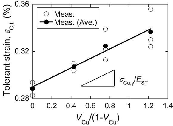
Fig. 8 Plot of the measured tolerant strain  $\varepsilon_{C,t}$  against  $V_{Cu}/(1-V_{Cu})$  for estimation of copper yield stress  $\sigma_{Cu,y}$ . The slope corresponds to  $\sigma_{Cu,y}/E_{ST}$  (eq. (9)).
