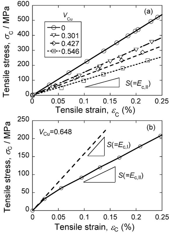
Fig. 2 Tensile stress  $\sigma_C$ -strain  $\varepsilon_C$  relation in the early stage up to  $\varepsilon_C = 0.25\%$  measured at 77 K for five specimens with  $V_{Cu} =$  (a) 0, 0.301, 0.427 and 0.546; and (b) 0.648. The results for the specimens with  $V_{Cu} = 0, 0.427$  and 0.546 were taken from a preceding work.<sup>2)</sup>
