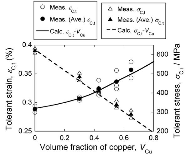
Fig. 7 Estimated values of tolerant strain  $\epsilon_{C,t}$  and tolerant stress  $\sigma_{C,t}$ , plotted against copper volume fraction ( $V_{Cu}$ ). The solid curve and broken line refer to the analyzed  $\epsilon_{C,t}-V_{Cu}$  and  $\sigma_{C,t}-V_{Cu}$  relations, respectively.
