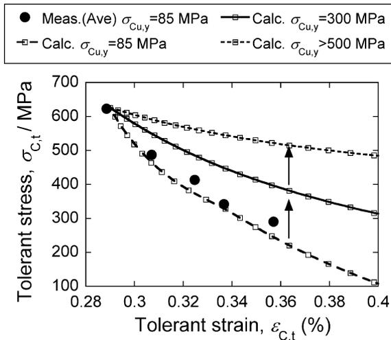
Fig. 9 Measured trade-off between tolerant stress  $\sigma_{C,t}$  and tolerant strain  $\varepsilon_{C,t}$  (closed circles) where  $\sigma_{Cu,y}$  was 85 MPa. Also shown are calculated relations for  $\sigma_{Cu,y} = 85$  MPa,  $\sigma_{Cu,y} = 300$  MPa and  $\sigma_{Cu,y} > 500$  MPa.
