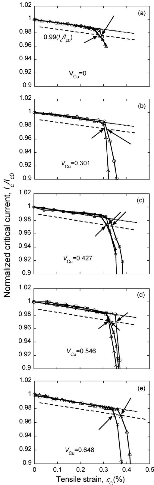
Fig. 6 Normalized critical current  $I_c/I_{c0}$ -tensile strain  $\epsilon_c$  relation as measured for specimens with  $V_{Cu} =$  (a) 0, (b) 0.301, (c) 0.427, (d) 0.546 and (e) 0.648. For each specimen, the strain tolerance  $\epsilon_{C,t}$  of critical current is indicated with an arrow.
