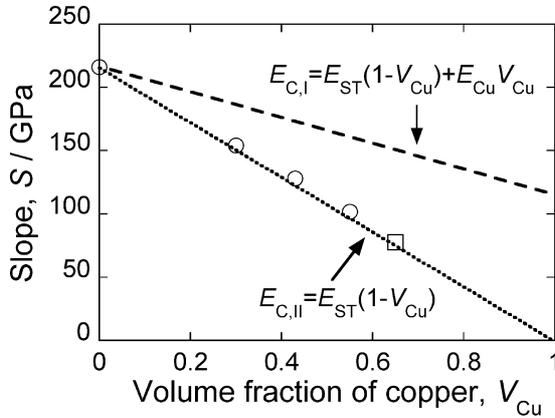
Fig. 3 Slope ( $S$ ) values (open circles) of the specimens with  $V_{Cu} = 0, 0.301, 0.427$  and 0.546 measured from the stress-strain curves in Fig. 2(a). The secondary modulus value  $E_{C,II}$  of the sample with  $V_{Cu} = 0.648$  in Fig. 2(b) is also shown with an open rectangle for reference. The  $E_{C,I}-V_{Cu}$  and  $E_{C,II}-V_{Cu}$  relations were calculated by the rule of mixtures (eqs. (1) and (2)) and are presented for comparison.
