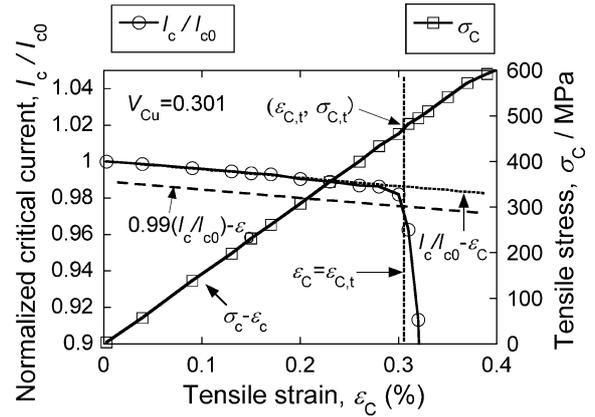
Fig. 5 Graphical representation for determining the tolerant strain  $\varepsilon_{C,t}$  and tolerant stress  $\sigma_{C,t}$  of critical current from measured  $I_c/I_{c0}-\varepsilon_C$  and  $\sigma_C-\varepsilon_C$  relations.
