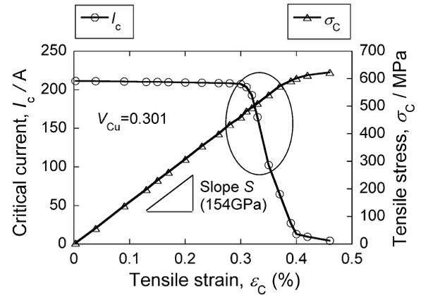
Fig. 1 An example of measured change in critical current  $I_c$  and tensile stress  $\sigma_C$  with increasing applied tensile strain  $\epsilon_C$ . The open circle shows the stress–strain range in which cracking of the superconducting layer initiates and extends, causing a reduction in critical current.
