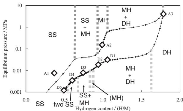
Fig. 5 Phase transformation for  $Ti_{1.0}V_{1.1}Mn_{0.9}$  along the  $P-C$  isotherm for the first absorption and desorption at 353 K. SS: solid-solution phase, MH: monohydride phase, DH: dihydride phase.
