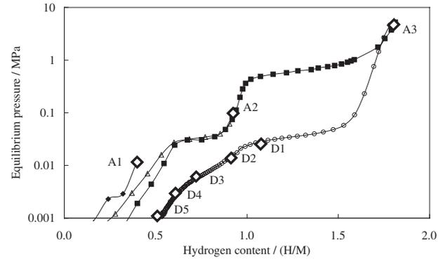
Fig. 1  $P$ - $C$  isotherms of  $\text{Ti}_{1.0}\text{V}_{1.1}\text{Mn}_{0.9}$ , measured at 353 K, for preparing hydride samples.
