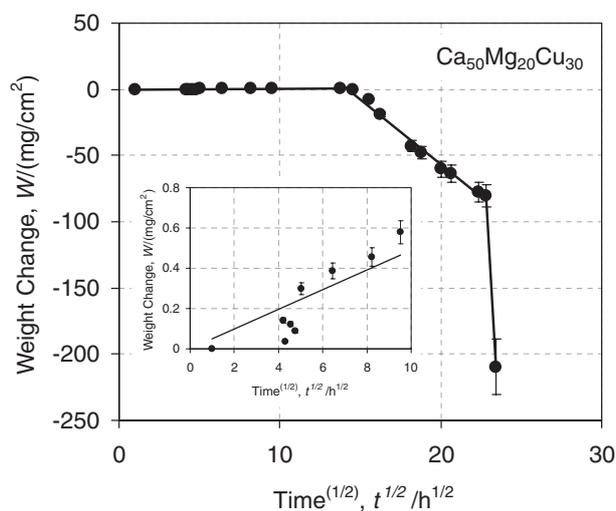
Fig. 3 Weight change per unit surface area of a ternary  $\text{Ca}_{50}\text{Mg}_{20}\text{Cu}_{30}$  metal glass versus square root of holding time in distilled water. Insert shows behavior during the first 100 hours of holding in water.
