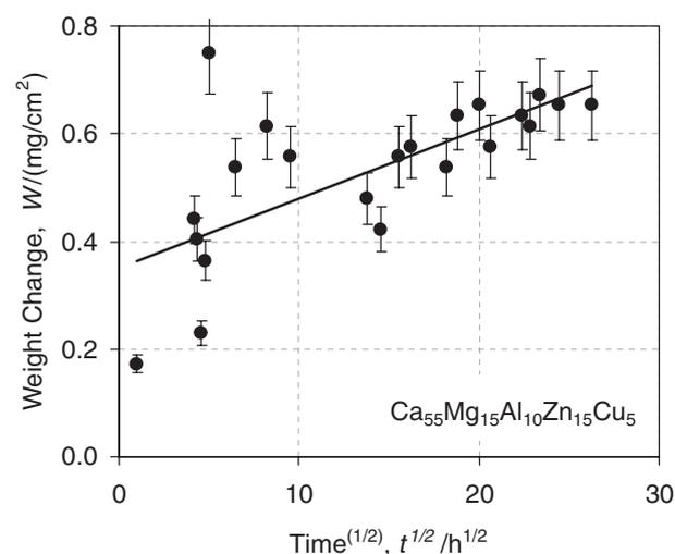
Fig. 6 Weight change per unit surface area of a  $\text{Ca}_{55}\text{Mg}_{15}\text{Al}_{10}\text{Zn}_{15}\text{Cu}_5$  metal glass versus square root of holding time in distilled water.
