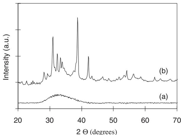
Fig. 1 X-ray diffraction patterns of  $\text{Ca}_{50}\text{Mg}_{20}\text{Cu}_{30}$  amorphous plates after (a) grinding and polishing with cooling water and oil and (b) after dry grinding and polishing. A broad halo is seen in figure (a), indicating amorphicity at the surface of the sample polished with low pressure and low heat; while both the amorphous halo and crystalline peaks are seen in figure (b).
