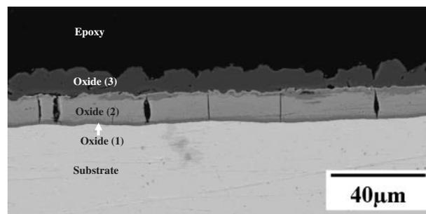
Fig. 5 SEM backscatter image of a near surface region of a  $\text{Ca}_{55}\text{Mg}_{18}\text{Zn}_{11}\text{Cu}_{16}$  amorphous sample after corrosion in distilled water for 2100 hours. The bright region at the bottom represents an image of a non-oxidized sample, above which three oxide layers are seen, which are identified by different gray levels.
