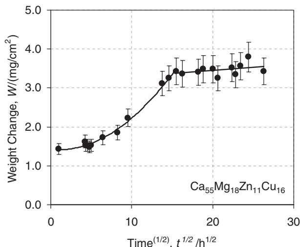
Fig. 4 Weight change per unit surface area of a  $\text{Ca}_{55}\text{Mg}_{18}\text{Zn}_{11}\text{Cu}_{16}$  metal glass versus square root of holding time in distilled water.
