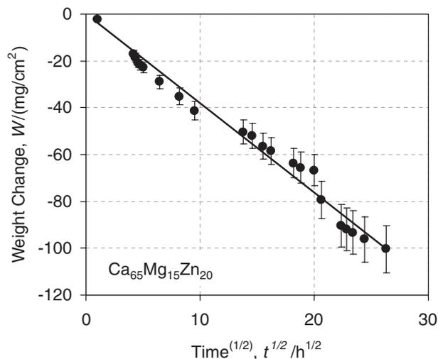
Fig. 2 Weight change per unit surface area of a ternary  $\text{Ca}_{65}\text{Mg}_{15}\text{Zn}_{20}$  metal glass versus square root of holding time in distilled water. The weight loss can be fit by a parabolic time dependence,  $W_1 = -a_1 t^{0.5}$ , where  $a_1 = 1.06 \times 10^{-3} \text{ mg}/(\text{cm}^2 \text{ s}^{0.5})$  is a rate constant.
