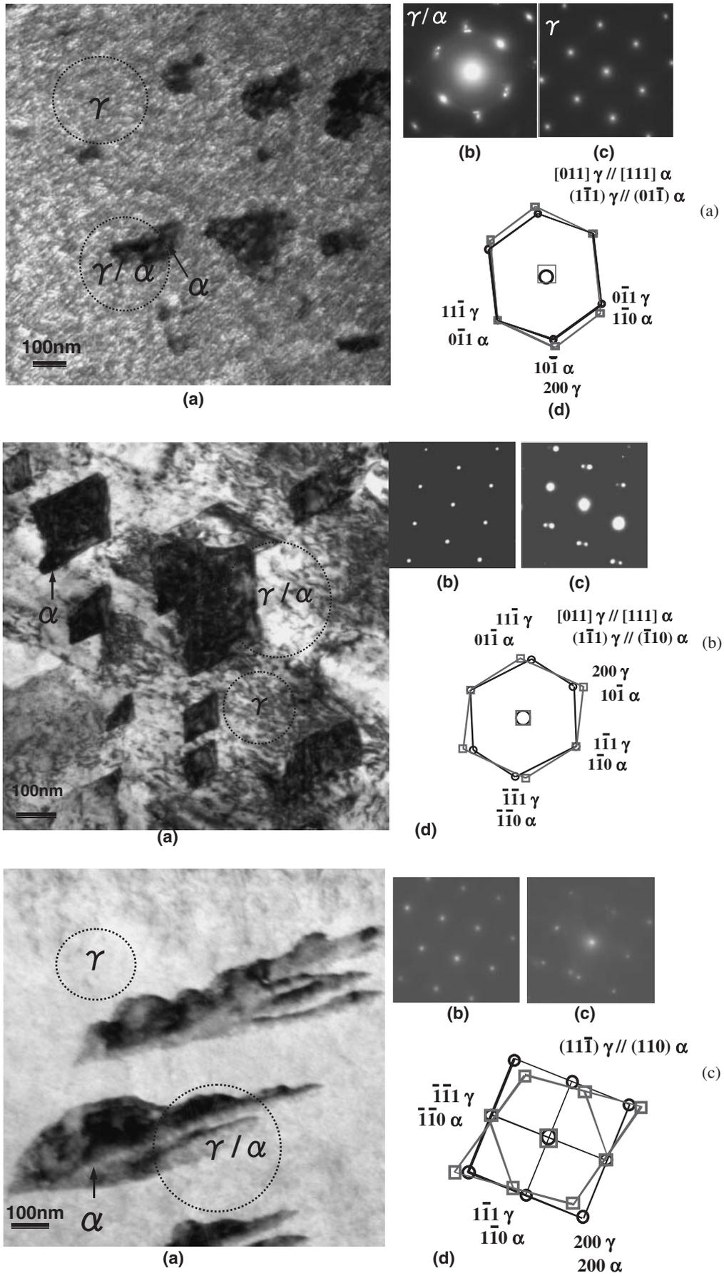
Fig. 2 Analysis of transformed phases by selected area diffraction after ion implantation with  $5 \times 10^{20}$  ions/m<sup>2</sup> at room temperature; (a) Fe<sup>+</sup> implantation (b) Ti<sup>+</sup> implantation and (c) Ar<sup>+</sup> implantation.
