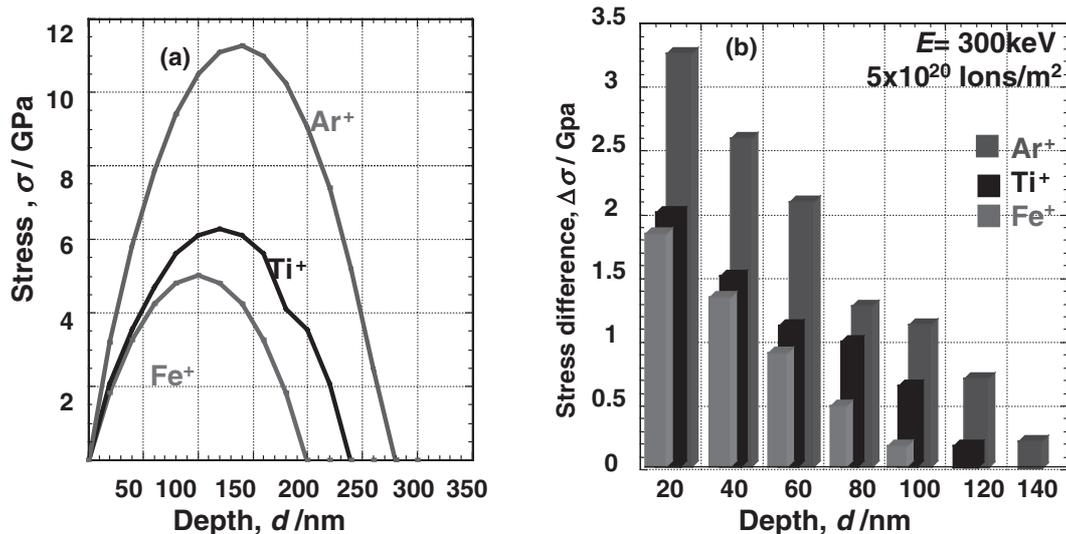
Fig. 7 Stress distribution profiles estimated from ion concentration implanted (a) and stress difference estimated from stress contribution profile in (b) at a given depth in the region with 20 nm width.
