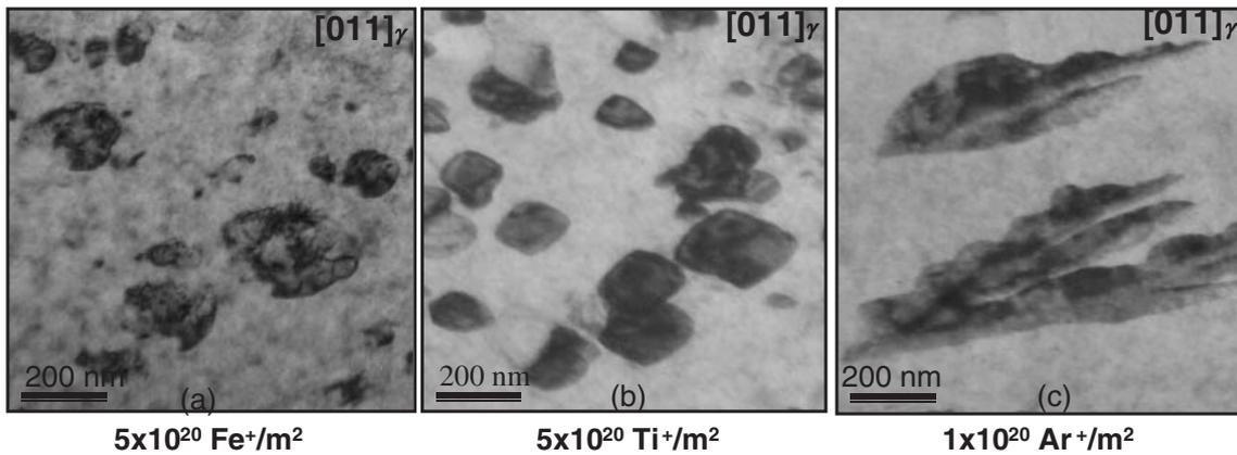
Fig. 1 Microstructures of the transformed phases after ion implantation with  $\text{Fe}^+$ ,  $\text{Ti}^+$  and  $\text{Ar}^+$  to the fluence of (a)  $5 \times 10^{20} \text{Fe}^+/\text{m}^2$ , (b)  $5 \times 10^{20} \text{Ti}^+/\text{m}^2$  and (c)  $1 \times 10^{20} \text{Ar}^+/\text{m}^2$  at room temperature.
