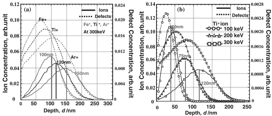
Fig. 4 Calculated profiles of concentration of implanted ions and the induced defects as a function of depth; (a) for the implantation with  $Fe^+$ ,  $Ti^+$  and  $Ar^+$  at 300 keV, and (b) for the implantation with  $Ti^+$  at 100 keV, 200 keV and 300 keV.
