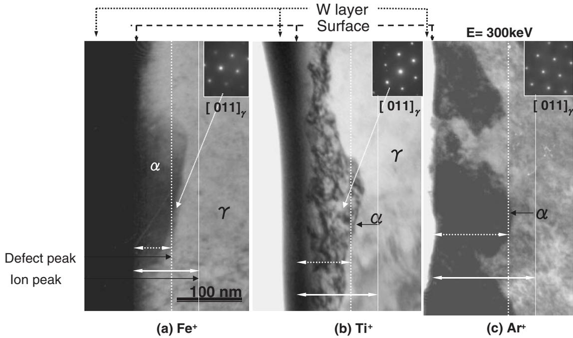
Fig. 5 Cross-sectional observation of microstructure of transformed phase after implantation with 300 keV: by (a) Fe<sup>+</sup>, (b) Ti<sup>+</sup> and (c) Ar<sup>+</sup>.
