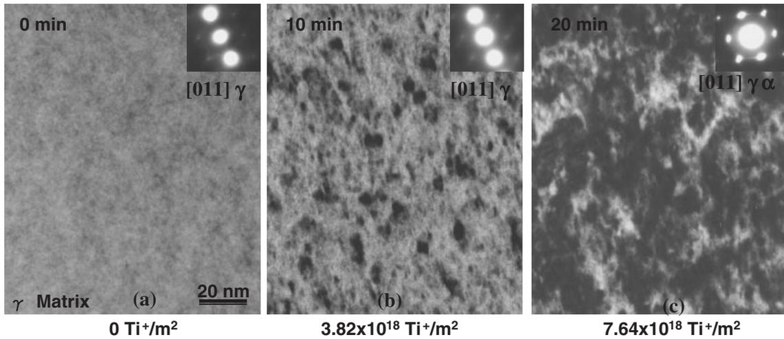
Fig. 3 Microstructural change during  $Ti^+$  ion implantation at room temperature with near the  $[011]_{\gamma}$  zone axis; (a) before ion implantation, (b) defect cluster formation, and (c) initiation of martensite transformation.
