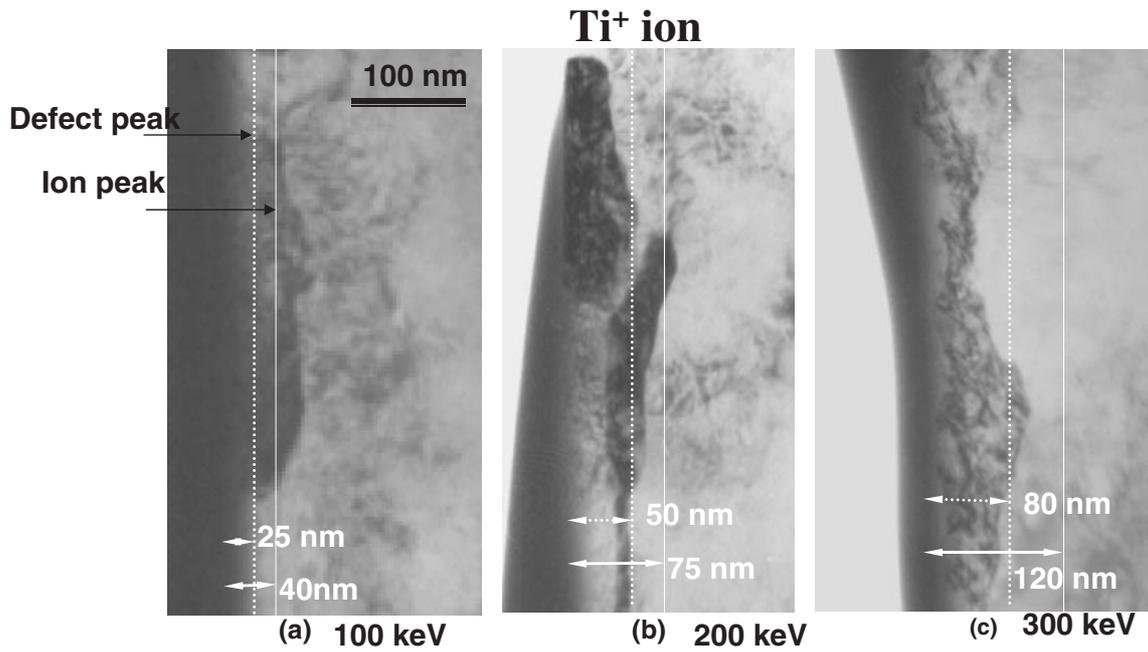
Fig. 6 Cross-sectional observation of transformed phase after Ti<sup>+</sup> implantation (a) at 100 keV, (b) at 200 keV and (c) at 300 keV.
