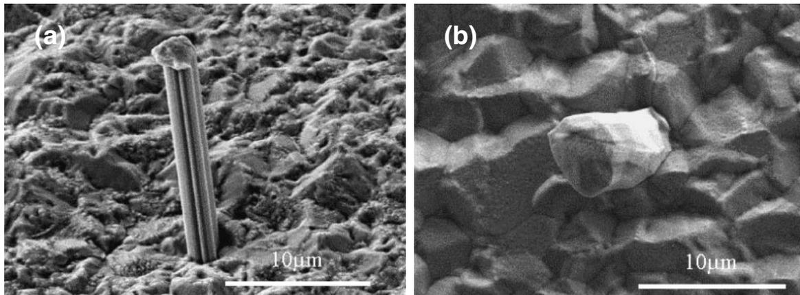
Fig. 2 (a) An enlarged SEM image of a long whisker on the eutectic SnCu finish is shown. (b) On the pure or matte Sn finish surface, short whiskers were observed as shown.
