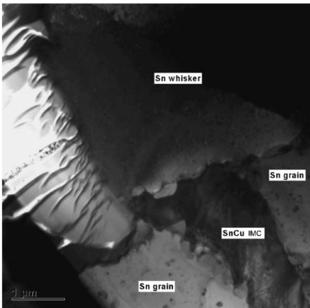
Fig. 9 Focused ion beam preparation of cross-section TEM samples.
