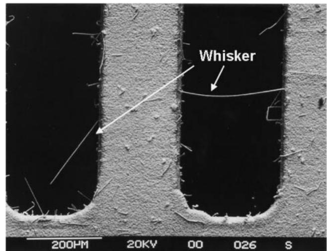
Fig. 1 An SEM image of Sn whiskers grown on a eutectic SnCu finished Cu leadframe.
