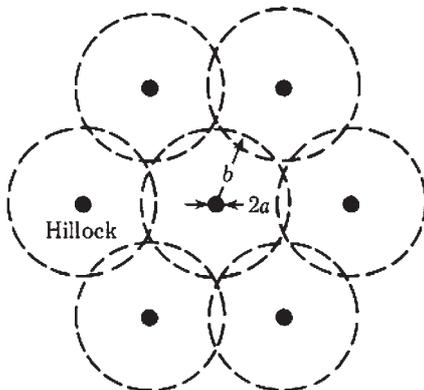
Fig. 11 Schematic diagram depicting a 2-dimensional distribution of Sn whiskers.
