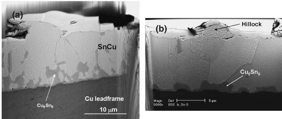
Fig. 4 (a) A higher magnification image of the interface between the SnCu and Cu layers, prepared by focused ion beam. Grain boundary precipitates of  $\text{Cu}_6\text{Sn}_5$  are shown. (b) Same kind of image of the interface between matte Sn and Cu. A much less grain boundary precipitates is found.
