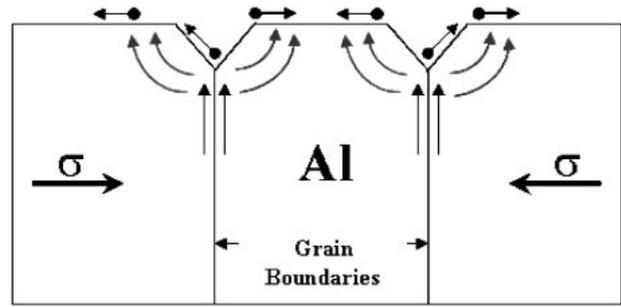
Fig. 6 A schematic diagram to show that when the surface has no oxide, the relaxation of stress can occur in each of the grains by atomic diffusion to the free surface of each grain.
