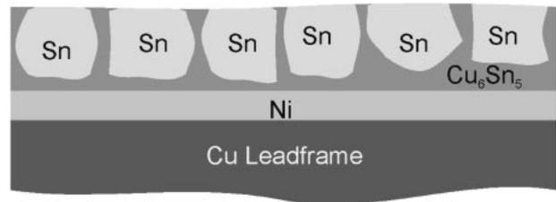
Fig. 12 A schematic diagram of the cross-section of a layer of Sn–2 to 5 mass%Cu finish plated on a Cu leadframe. The Sn grains in the finish are surrounded by grain boundary precipitates of  $\text{Cu}_6\text{Sn}_5$ .
