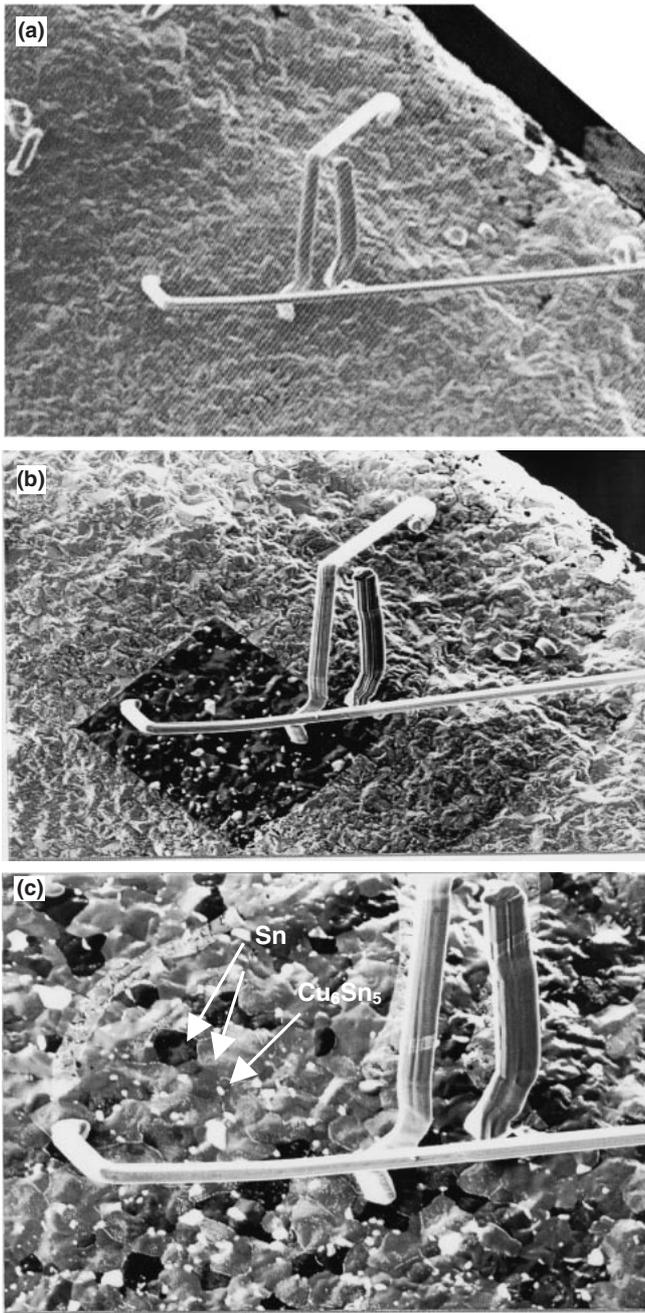
Fig. 7 (a) A focused ion beam image of a group of whiskers on the SnCu finish is shown. (b) The oxide on a rectangular area of the surface of the finish was sputtered away by using a glancing incidence ion beam to expose the microstructure beneath the oxide. (c) A higher magnification image of the sputtered area is shown, in which the microstructure of Sn grains and grain boundary precipitates of  $\text{Cu}_6\text{Sn}_5$  are clear.
