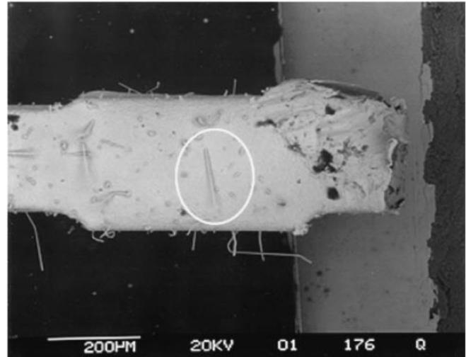
Fig. 10 Cross-sectional TEM image of the root of a Sn whisker.
