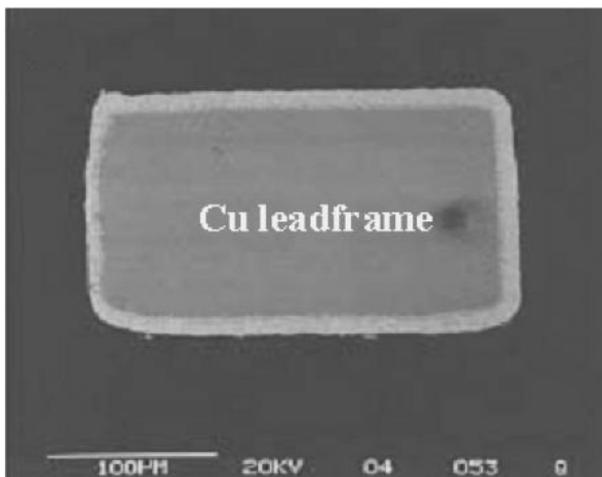
Fig. 3 Cross-sectional SEM image of a leadframe leg with SnCu finish is shown.
