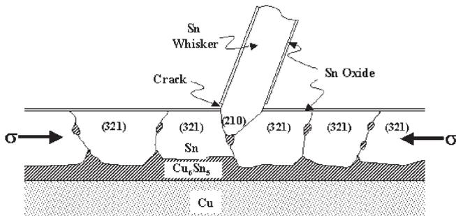
Fig. 5 We consider a fixed volume “ $V$ ” in the Sn finish that contains a grain boundary precipitate of IMC and the stress induced due to the interdiffusion of a Cu atom.
