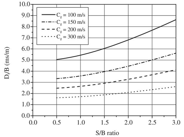
Fig. 17 Variation in the optimum fragmentation condition with various gas flow velocities.
