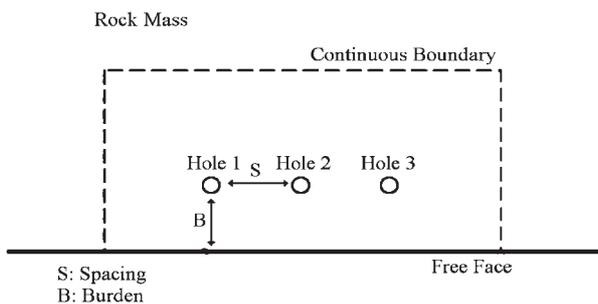
Fig. 1 Analysis model for bench blast simulation.
