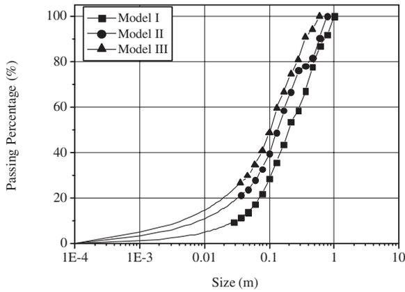
Fig. 9 Variation of the fragmentation with specific charge increase.
