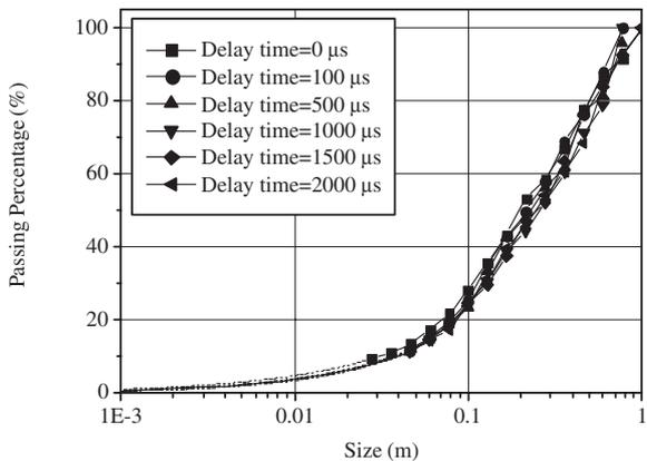
Fig. 14 Size distributions on a log-lin with the variation of delay time between holes.
