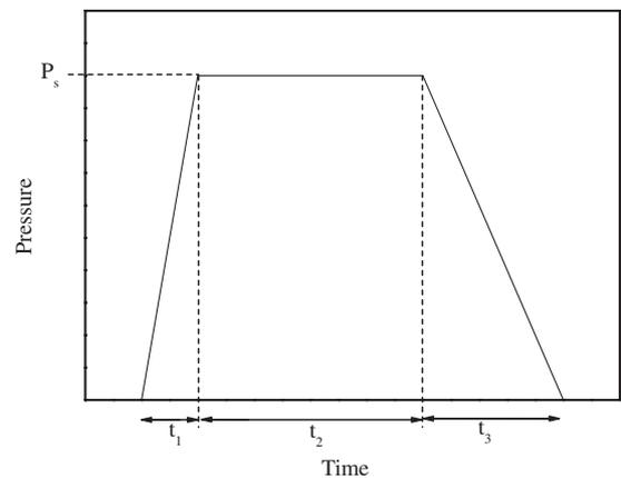
Fig. 3 Pressure-time history for gas pressure in the boreholes.
