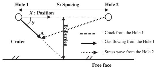
Fig. 16 Scheme diagram representing the interaction between gas flow and the stress wave from the adjacent hole.
