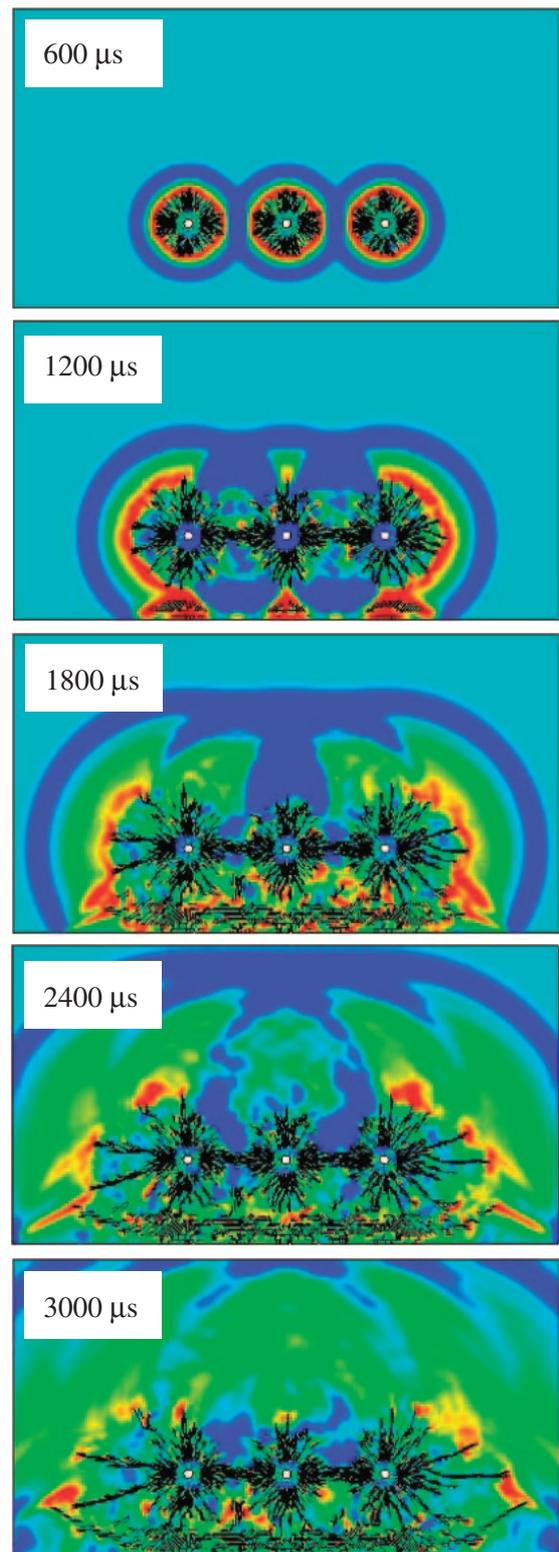
Fig. 4 Maximum principal stress distribution and crack propagation in Model I.
