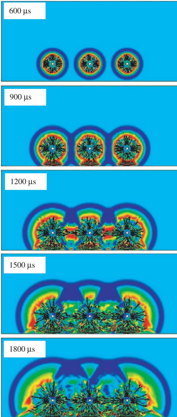
Fig. 11 Maximum principal stress distribution and crack propagation in a wide space blast model.
