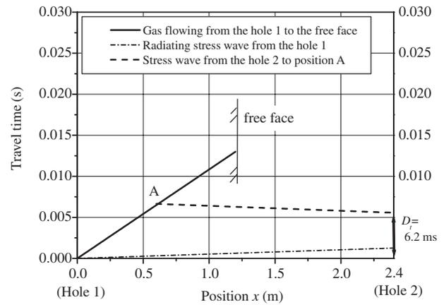
Fig. 18 Determining the practical optimum delay time for Model I used.
