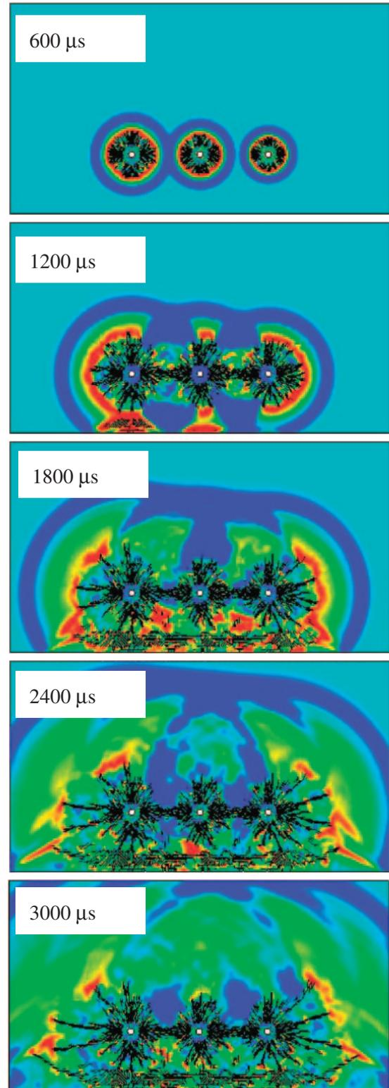
Fig. 13 Maximum principal stress distribution and crack propagation in a Type I with 100 μs delay timing interval.
