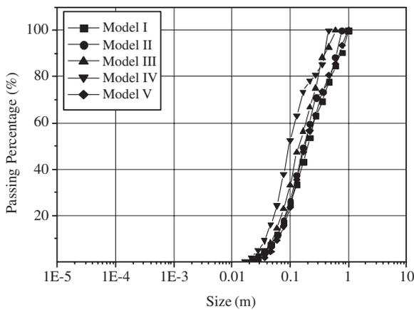
Fig. 7 Numerical fragment size distributions obtained by image analysis.
