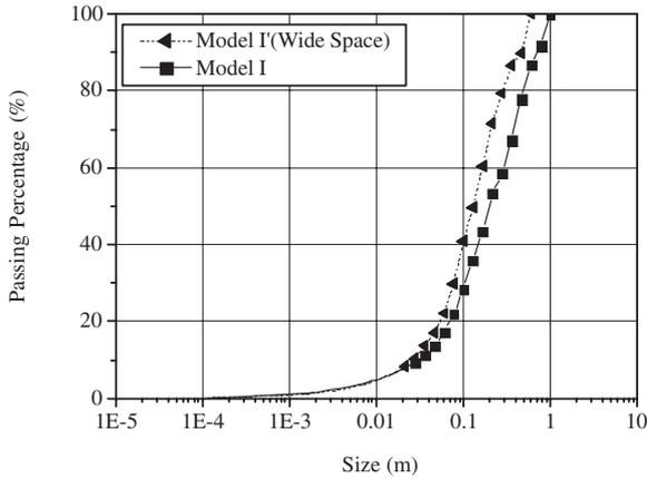
Fig. 12 Comparison of fragmentation in general bench blast and wide space pattern.
