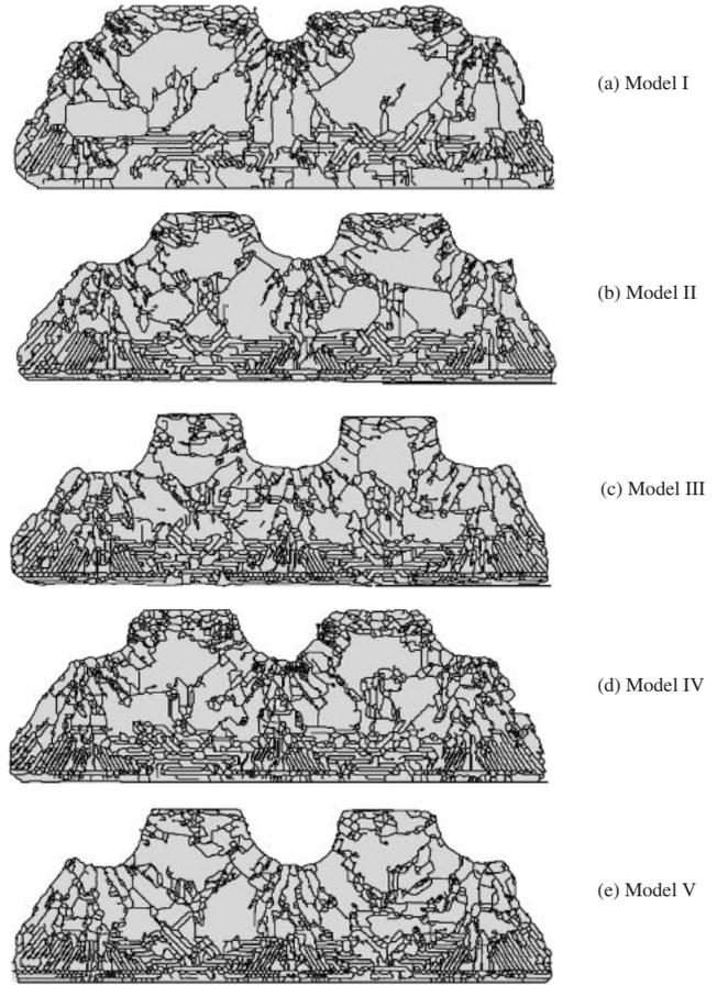
Fig. 6 Automatic delineation results for the fragment size calculations.
