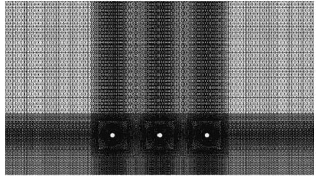
Fig. 2 Finite element layout for the analysis models.
