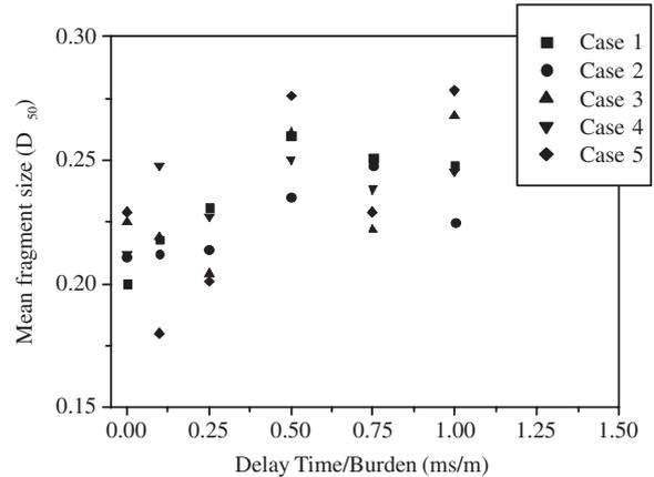
Fig. 15 Variation of average size with the ratio of delay time and burden.
