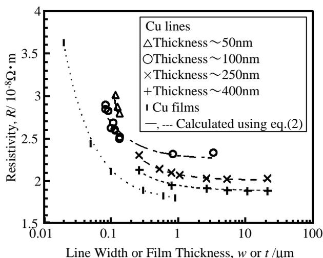
Fig. 4 Resistivity of Cu samples (as a function of line width).
