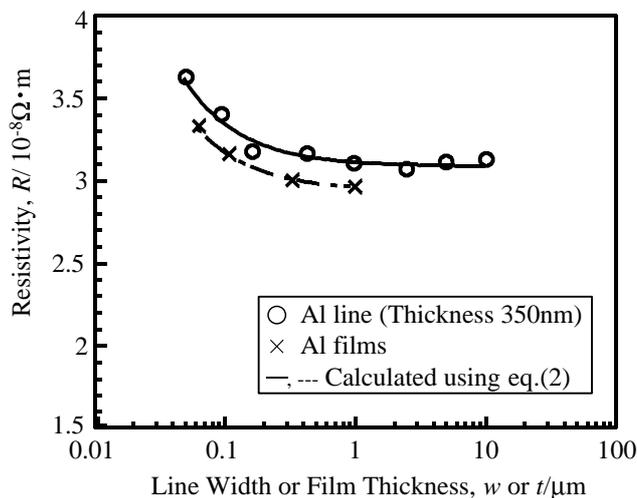
Fig. 5 Resistivity of Al samples (as a function of line width).
