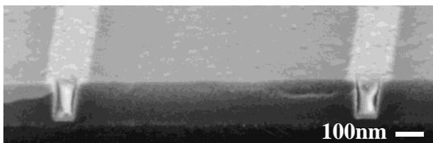
Fig. 1 SEM micrograph of 70-nm-wide Cu lines.
