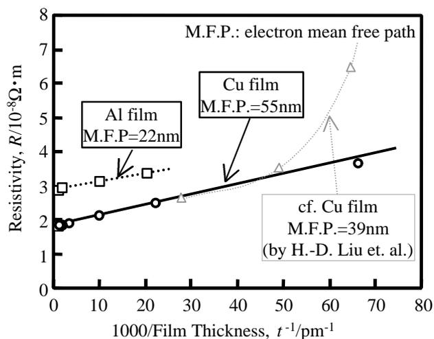
Fig. 2 Resistivity values as a function of film thickness.
