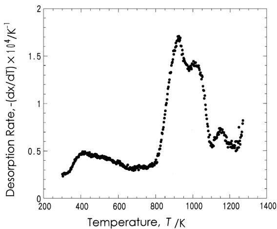
Fig. 5 A thermal desorption spectrum observed after quenching from the bcc ( $\alpha$ ) phase. The heat treatment was made at 1.8 GPa, 870 K for 3 h. Measurements were made at 20 min after recovery to ambient condition.
