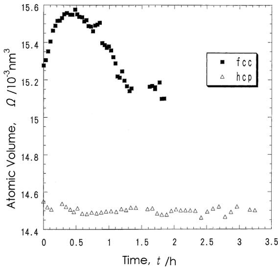
Fig. 4 Atomic volume (volume per Cr atom) of fcc ( $\gamma$ ) and hcp ( $\epsilon$ ) hydride as a function of holding time at 1170 K,  $p(\text{H}_2) = 2.6$  GPa and 5 GPa, respectively.
