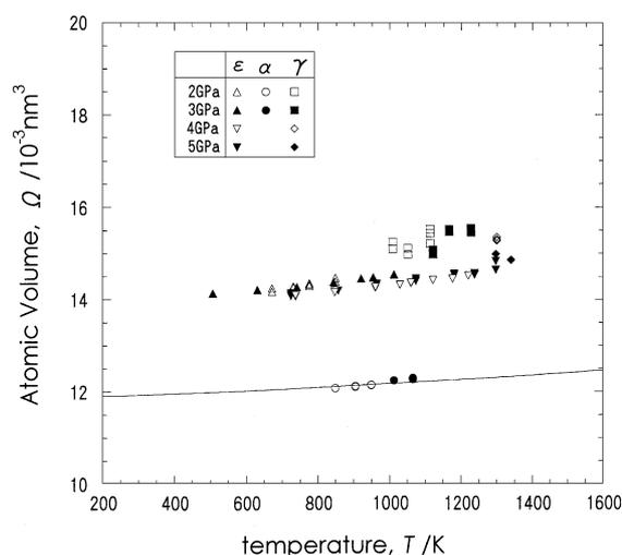
Fig. 2 Temperature dependence of the atomic volume (volume per Cr atom) at four different hydrogen pressures, encompassing three different phases; bcc ( $\alpha$ ), hcp ( $\epsilon$ ) and fcc ( $\gamma$ ). A curve drawn in the lower part of the Figure represent the thermal expansion of metallic Cr at ambient pressure.<sup>29)</sup>
