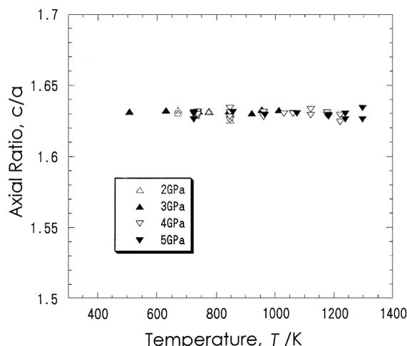
Fig. 3 Temperature dependence of the axial ratio of the hcp phase ( $\epsilon$ ) at four different hydrogen pressures.
