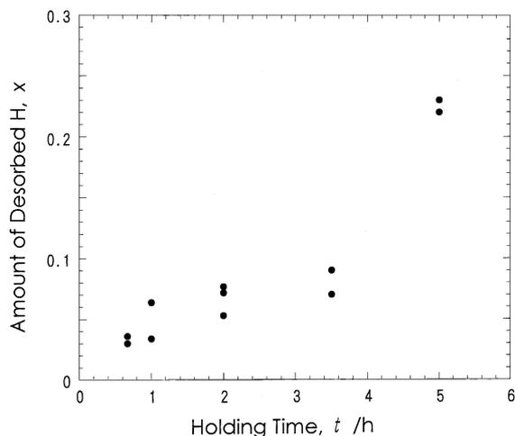
Fig. 8 The amount of hydrogen desorbed after heat treatments in the fcc phase (1.8 GPa, 1170 K) for variable lengths of time. The amounts desorbed between 450 K and 750 K have been included.
