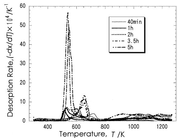
Fig. 7 Thermal desorption spectra observed after heat treatments in the fcc ( $\gamma$ ) phase. The heat treatments were performed at 1.8 GPa, 1170 K for 40 min, 1 h, 2 h, 3.5 h and 5 h. The measurements were made at various times after recovery.
