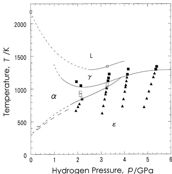
Fig. 1 Phase diagram of the Cr-H system as a function of hydrogen pressure and temperature. The crystal structures are; bcc ( $\alpha$ ), hcp ( $\epsilon$ ) and fcc ( $\gamma$ ). In the lower  $p$ ,  $T$  region, a cross has been taken from Ref. 6), and a broken line from Ref. 7).
