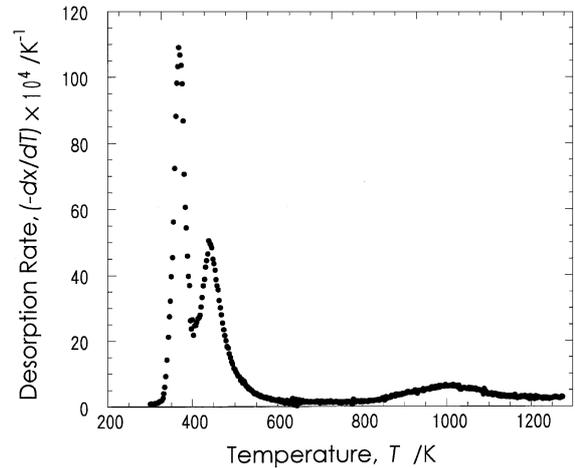
Fig. 6 A thermal desorption spectrum observed after quenching from the hcp ( $\epsilon$ ) phase. The heat treatment was made at 4.4 GPa, 1070 K for 15 min, and the measurement was made 33 min after recovery.
