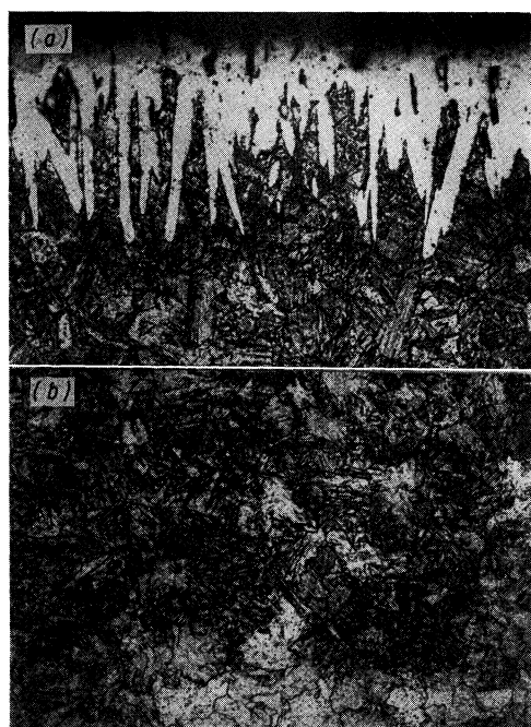
Photo.1 Microstructure of the boro-carburized layer on iron immersed in a hot bath consisting of 27% B_4C , 7% BaO, 33% KCl, and 33% NaCl at 1000°C for 6 hr. (a) surface, (b) interface between matrix and carburized layer.
