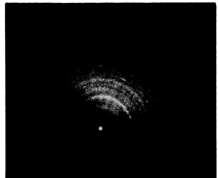
Photo.2 Electron diffractogram of the anodic film. pH=2, H_2SO_4, Total SO_4^{2-}=2.5 \times 10^{-1} mol/l, Br^- concent = 5 \times 10^{-1} mol/l, Temp. = 25^\circ C, Set potential=0.6 V, Time=30 min
