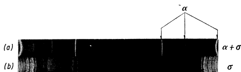
Photo.6 X-ray Debye-Scherrer patterns of \sigma -phase (a) particles (55 at% Cr-Fe) (b) bulk (50 at% Cr-Fe)
