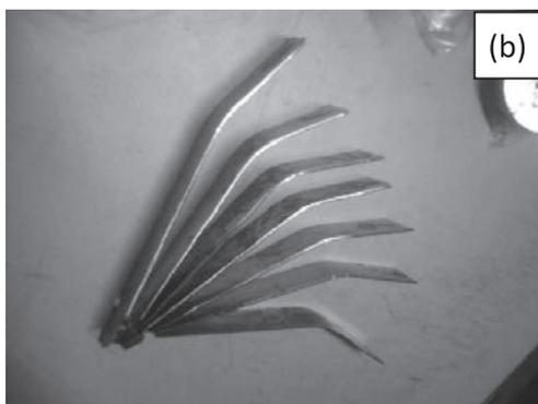
Fig. 3 The mechanical properties of samples prepared by high vacuum die-casting (a) typical three-point bending stress-strain curve of samples with different thickness (b) some plastic samples after three-point bending test.
