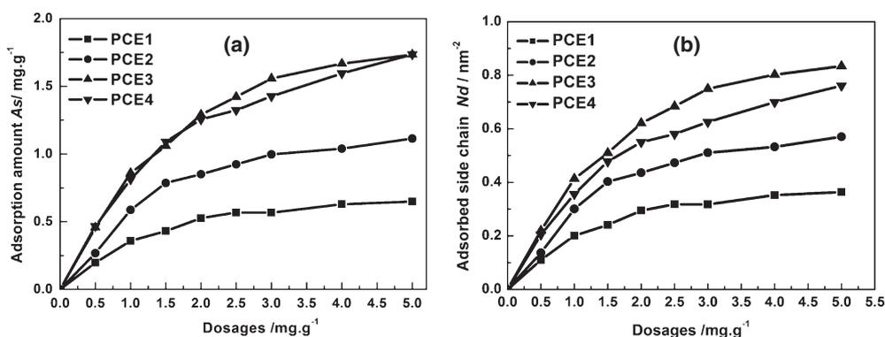
Fig. 2 Adsorption amounts of PCE comb-like copolymers on cement surface (a) and the adsorbed number of side chain per unit area of cement (b) as a function of the amount of PCE introduced.
