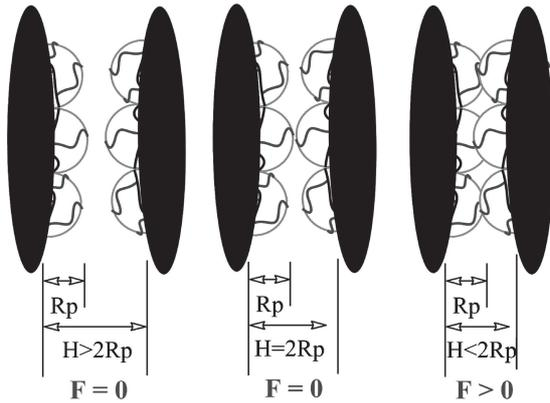
Fig. 5 Schematic illustration of the steric repulsion hypothesis.<sup>14)</sup>
