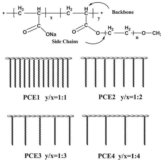
Fig. 1 Illustration of the chemical structure of comb-like copolymers with different graft densities.
