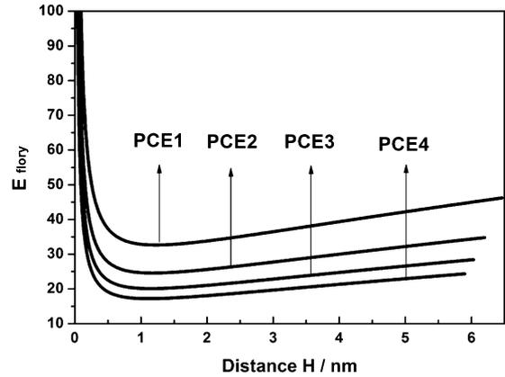
Fig. 6 The Flory energy of cement suspensions using PCE comb-like polymer with different grafting densities as dispersant.
