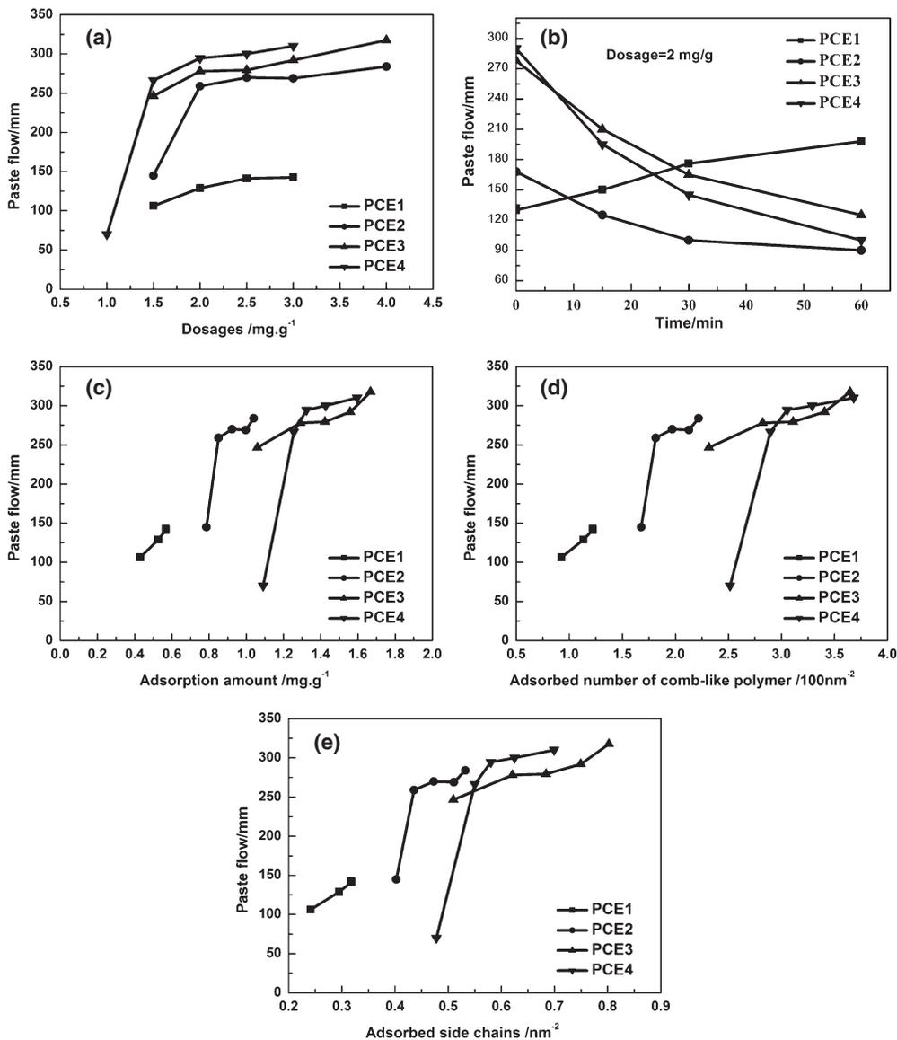
Fig. 3 Dispersion behavior of PCE with different grafting densities (a) dispersion vs. dosages, (b) dispersion vs. time, (c) dispersion vs. adsorbed amount, (d) dispersion vs. adsorbed number of comb-like polymers, and (e) dispersion vs. adsorbed side chains.
