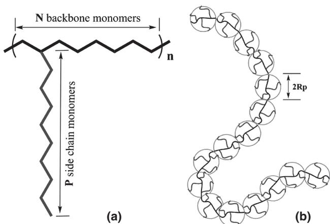
Fig. 4 (a) Schematic representation of the comb-like polymers considered. The polymer contains  $n$  segments, each segment contains one side chain which has  $P$  monomers and each segment contains  $N$  backbone monomers; (b) illustration of the conformation of flexible backbone worm (FBW).
