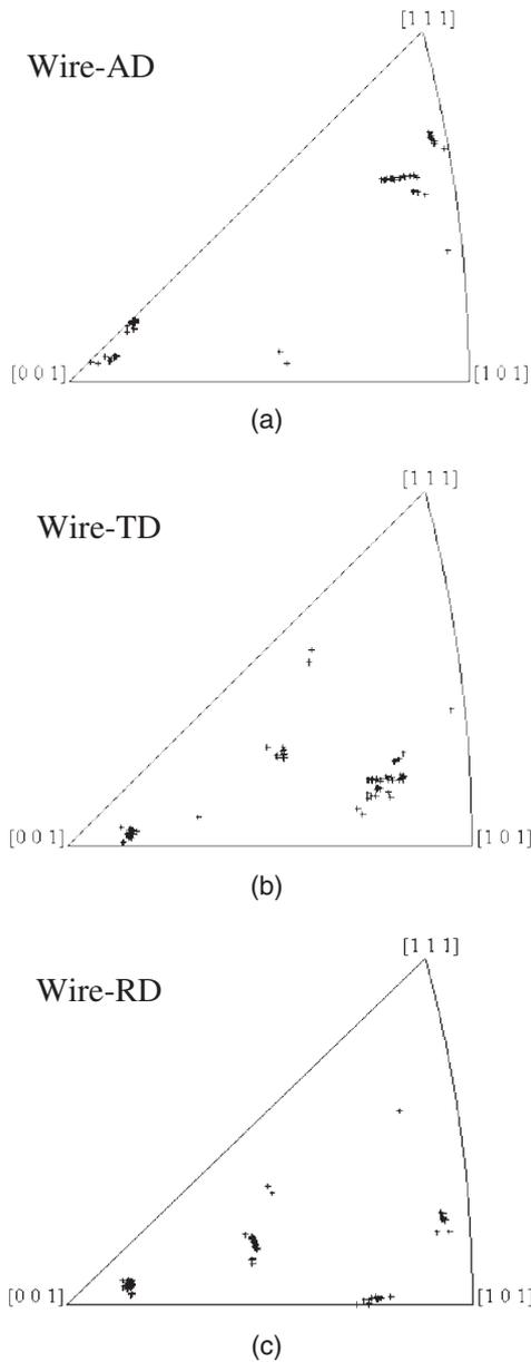
Fig. 8 IPF map of annealed wire: (a) AD, (b) TD and (c) RD.
