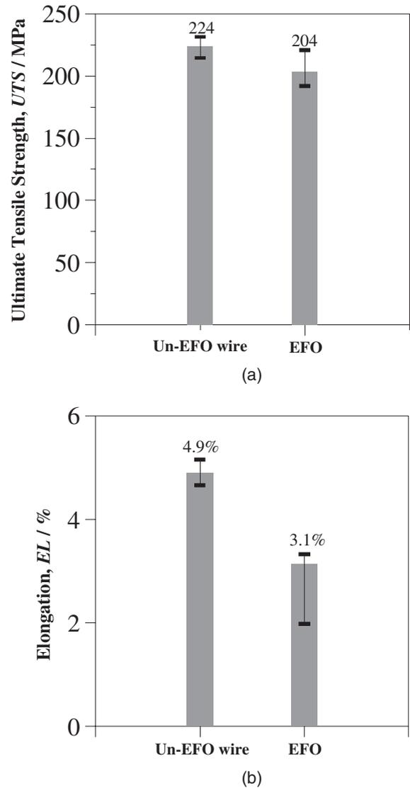
Fig. 5 Tensile mechanical properties of the 225 $^{\circ}\text{C}$  annealed wire before and after EFO process: (a) UTS and (b) EL.
