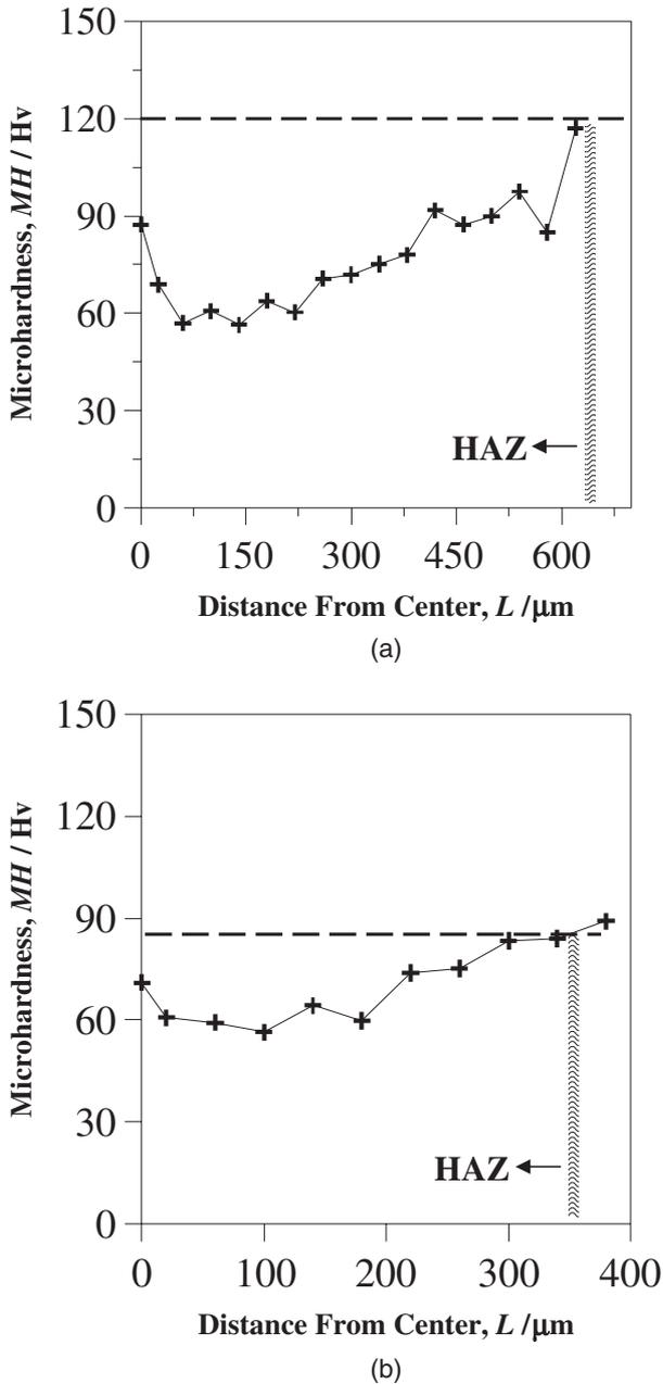
Fig. 4 Micro-hardness of the wire after EFO process (the origin of the cross axle is the center of FAB): (a) un-annealed wire and (b) 225 $^{\circ}\text{C}$  annealed (The dotted line is the average hardness value of the un-EFO wires).
