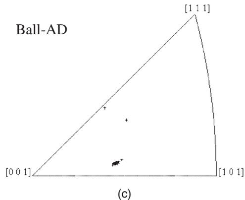
Fig. 10 IPF map of annealed wire on the ball: (a) AD, (b) TD and (c) RD.
