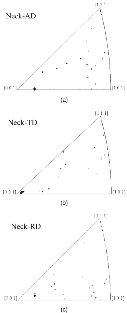
Fig. 9 IPF map of annealed wire on the neck: (a) AD, (b) TD and (c) RD.
