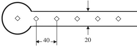
Fig. 1 The schematic illustration of the micro-hardness measuring. (unit:  $\mu\text{m}$ )
