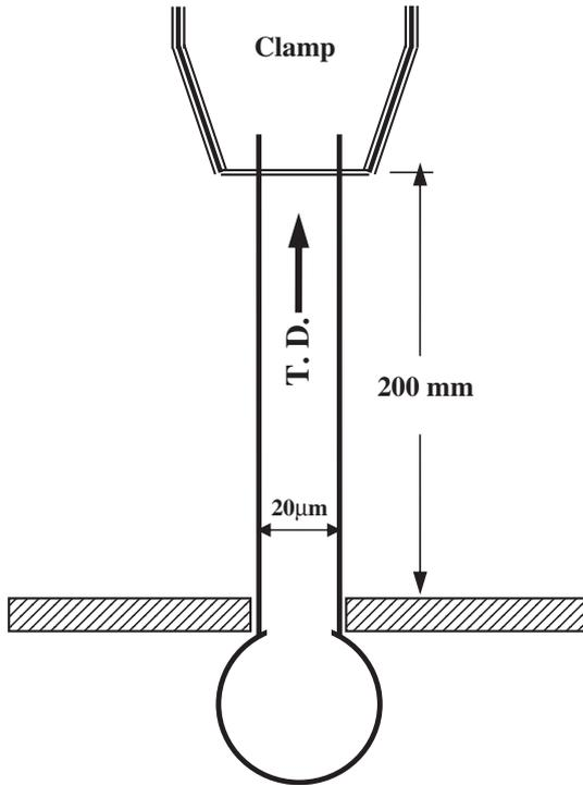
Fig. 2 The schematic illustration of the tensile testing for the neck.
