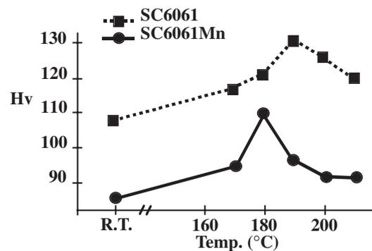
Fig. 11 Variation of microhardness values of SC6061 and SC6061Mn alloys with aging temperature (aging time: 2 hours).
