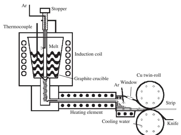
Fig. 1 Schematic drawing of the twin roll caster used in the present study.
