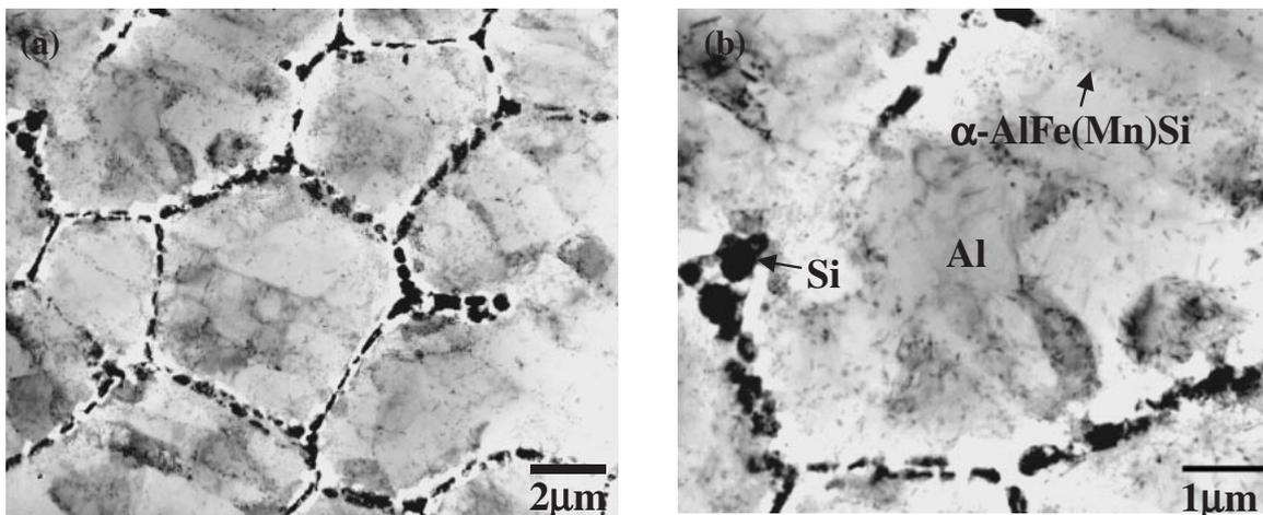
Fig. 6 (a) BF micrograph of as-cast SC6061Mn alloy and (b) magnified BF micrograph showing  $\alpha$ -AlFe(Mn)Si particles within Al matrix.
