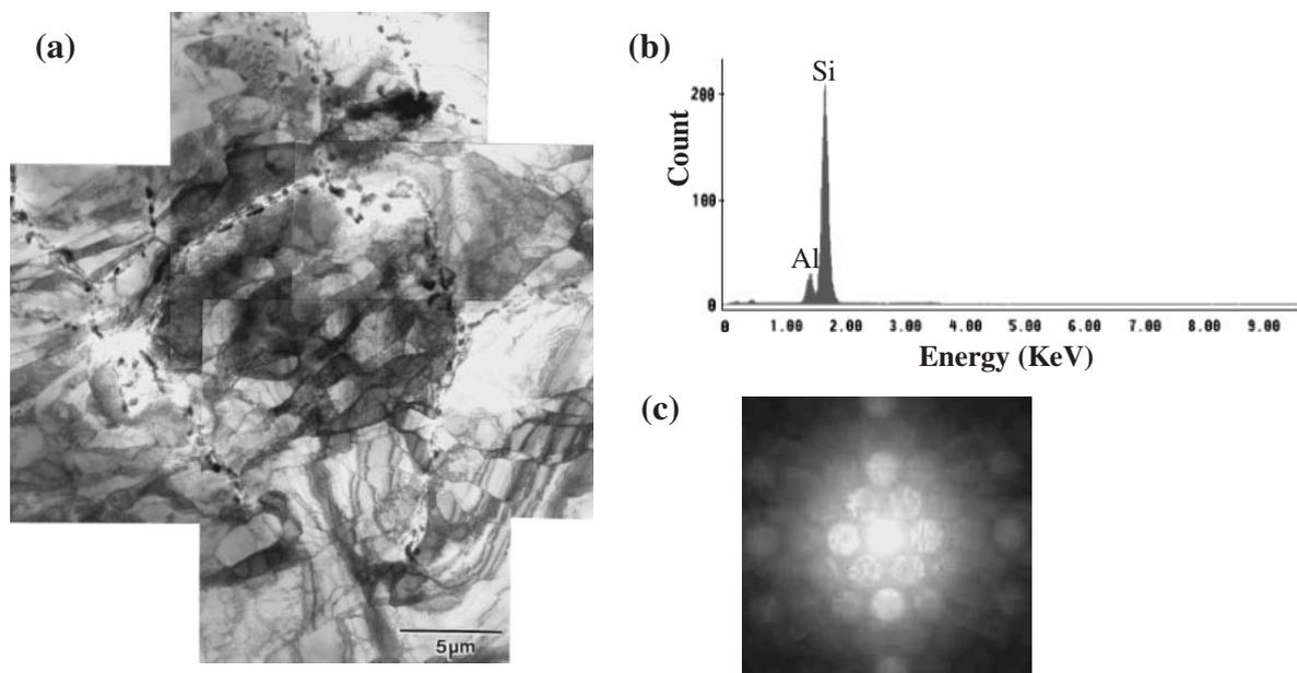
Fig. 4 (a) BF micrograph of as-cast SC6061 alloy, (b) EDS spectra from Si containing particles and (c) microdiffraction pattern of Si containing particles.
