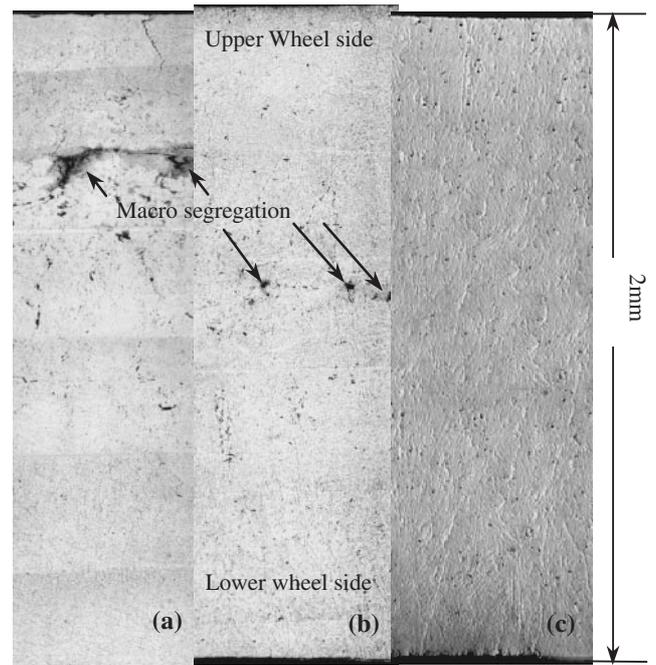
Fig. 2 Cross-sectional optical micrographs of as-cast SC6061 alloy processed with different roll speeds; (a) 16 m/min, (b) 8 m/min, and (c) 4 m/min.
