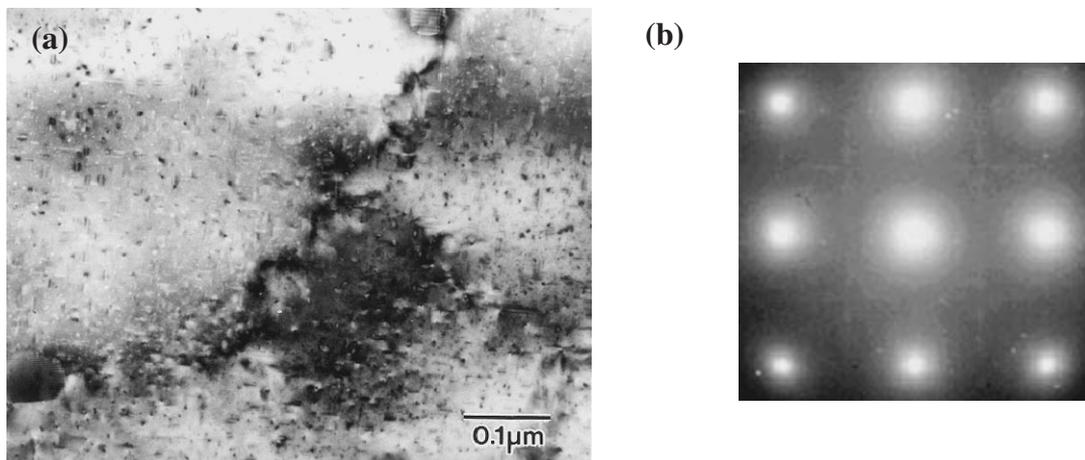
Fig. 8 (a) BF micrograph of T6 treated SC6061 alloy showing  $Mg_2Si$  particles within the Al matrix and (b) selected area diffraction pattern showing the streaks arising from  $Mg_2Si$  particles.
