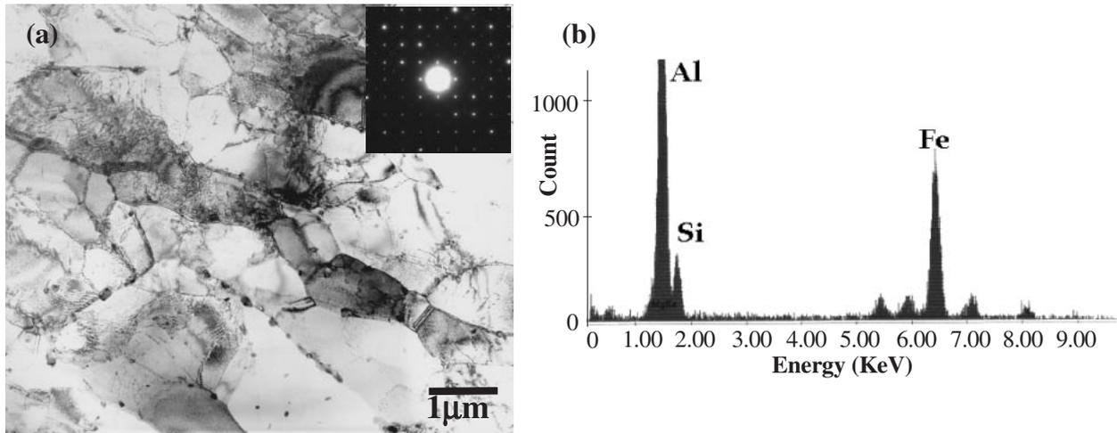
Fig. 7 (a) BF micrograph of T6 treated SC6061 alloy showing  $\alpha$ -AlFeSi particles along grain boundaries and (b) EDS spectra from an  $\alpha$ -AlFeSi particle.
