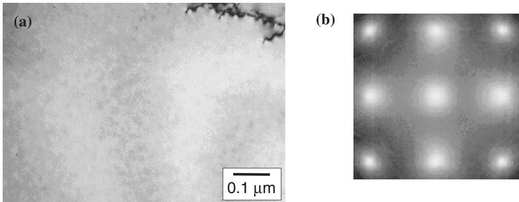
Fig. 10 (a) BF micrograph of T6 treated SC6061Mn alloy showing Al matrix and (b) selected area diffraction pattern.
