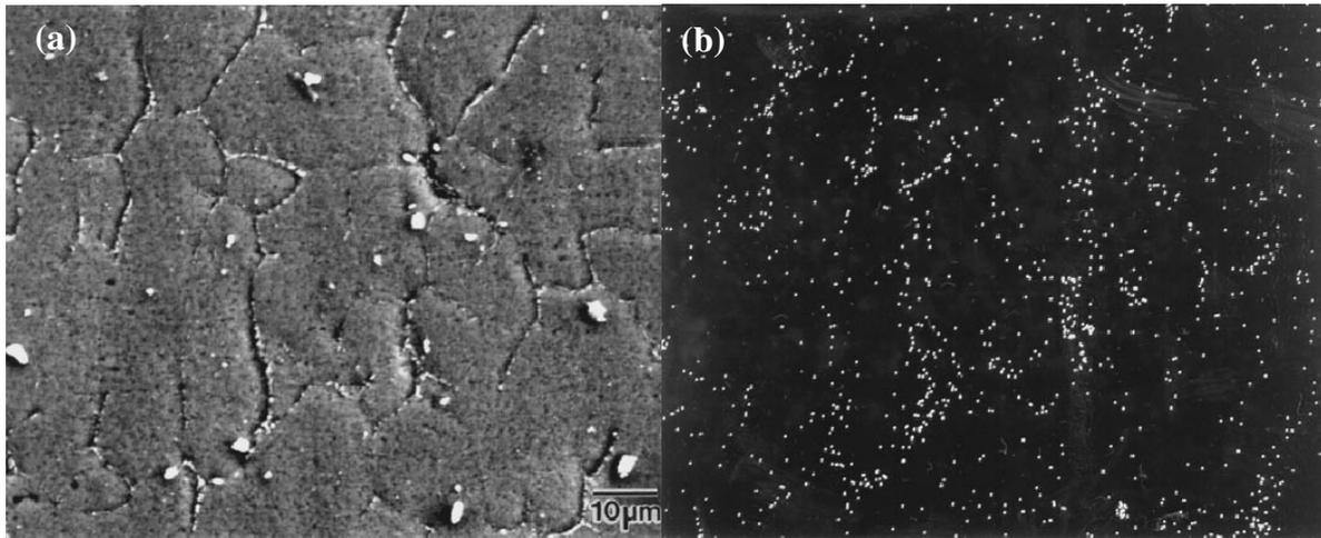
Fig. 3 SEM micrographs of as-cast SC6061 alloy showing the segregation of Si along grain boundaries; (a) SEM image and (b) X-ray mapped image.
