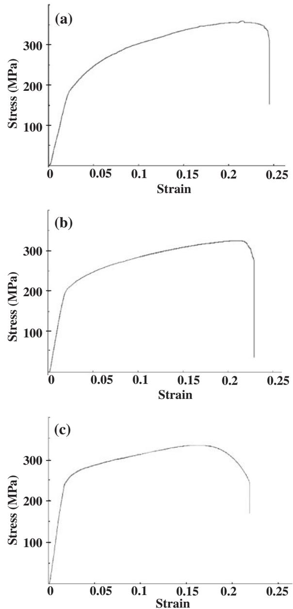
Fig. 12 Representative stress-strain curve of T6 treated specimens; (a) SC6061Mn alloy, (b) SC6061 alloy and (c) commercial IM6061 alloy.
