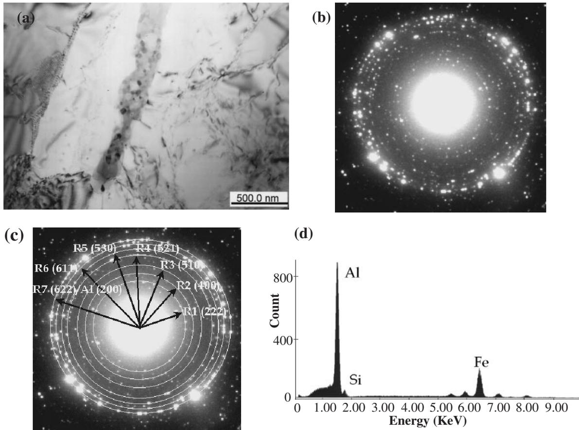
Fig. 5 (a) BF micrograph showing grain boundary particles in as-cast SC6061 alloy, (b) selected area diffraction pattern of grain boundary particles, (c) schematic drawing and indexing of selected area diffraction shown in (b), and (d) EDS spectra from grain boundary particles.
