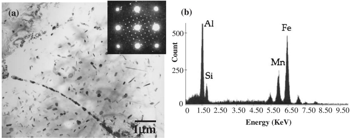
Fig. 9 (a) BF micrograph of T6 treated SC6061Mn alloy showing  $\alpha$ -AlFe(Mn)Si particles along grain boundaries and within the Al matrix and (b) EDS spectra from an  $\alpha$ -AlFe(Mn)Si particle.
